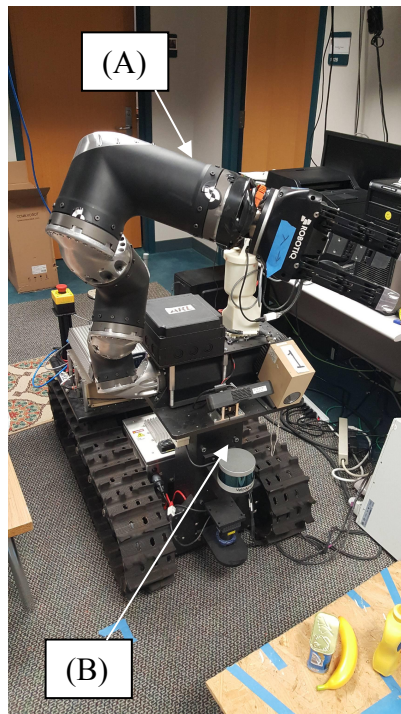
Figure 2: RoMan platform. This platform is equipped with a seven-degree-of-freedom arm, gripper, sensor suite, and capable of autonomously detecting and grasping objects
