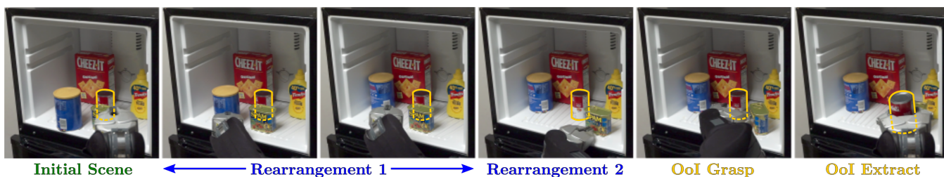
Fig. 7. A MAMO solution generated by M4M. The tomato soup can (yellow outline) is the OoI, all other objects are movable.
